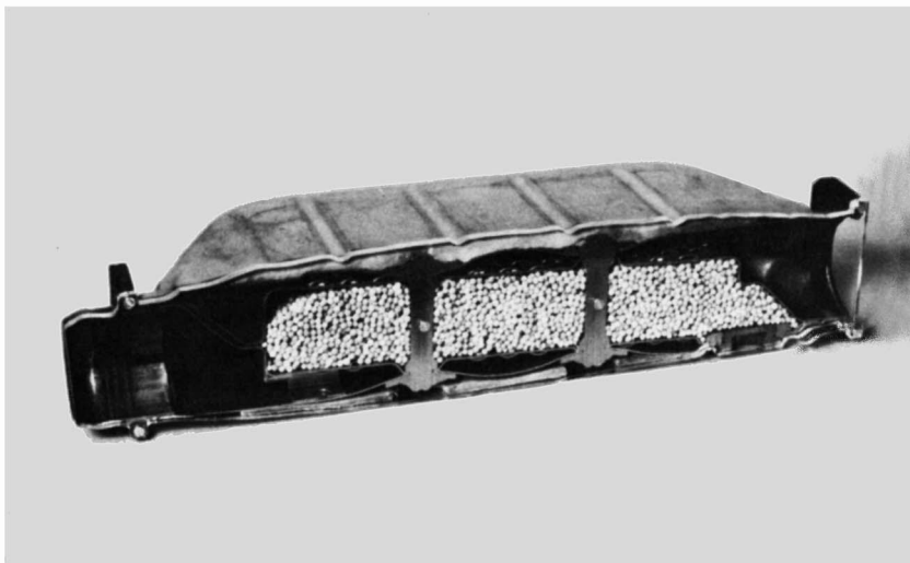
Figure 2 The catalytic converter for the complete combustion of automobile exhaust. It oxidizes unburned hydrocarbons, and carbon monoxide to carbon dioxide and water, and reduces nitrogen oxides to dinitrogen simultaneously
